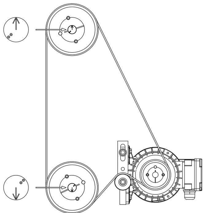
When the arrows at the end of the shafts are pointing in the opposite direction of each other, the short pivot arms will be approximately positioned like in the figure below:
