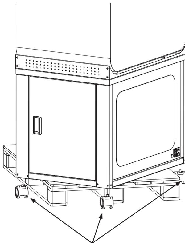
Slide the printer so three of the corners comes out from the pallet like shown above. Add the wheels on the three available corners. Then slide the printer carefully so the last corner comes outside the pallet. Add the last wheel. Lift the printer carefully down to the floor.
