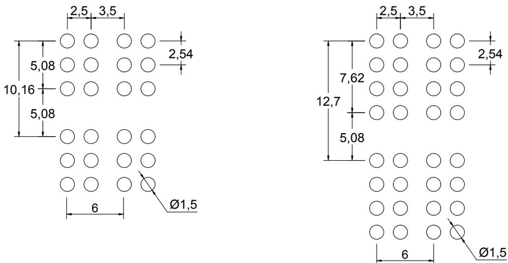
The drawing on this page is meant to help to understand the basic principle of how the dots are printed. Please also see the drawings on the next page.
