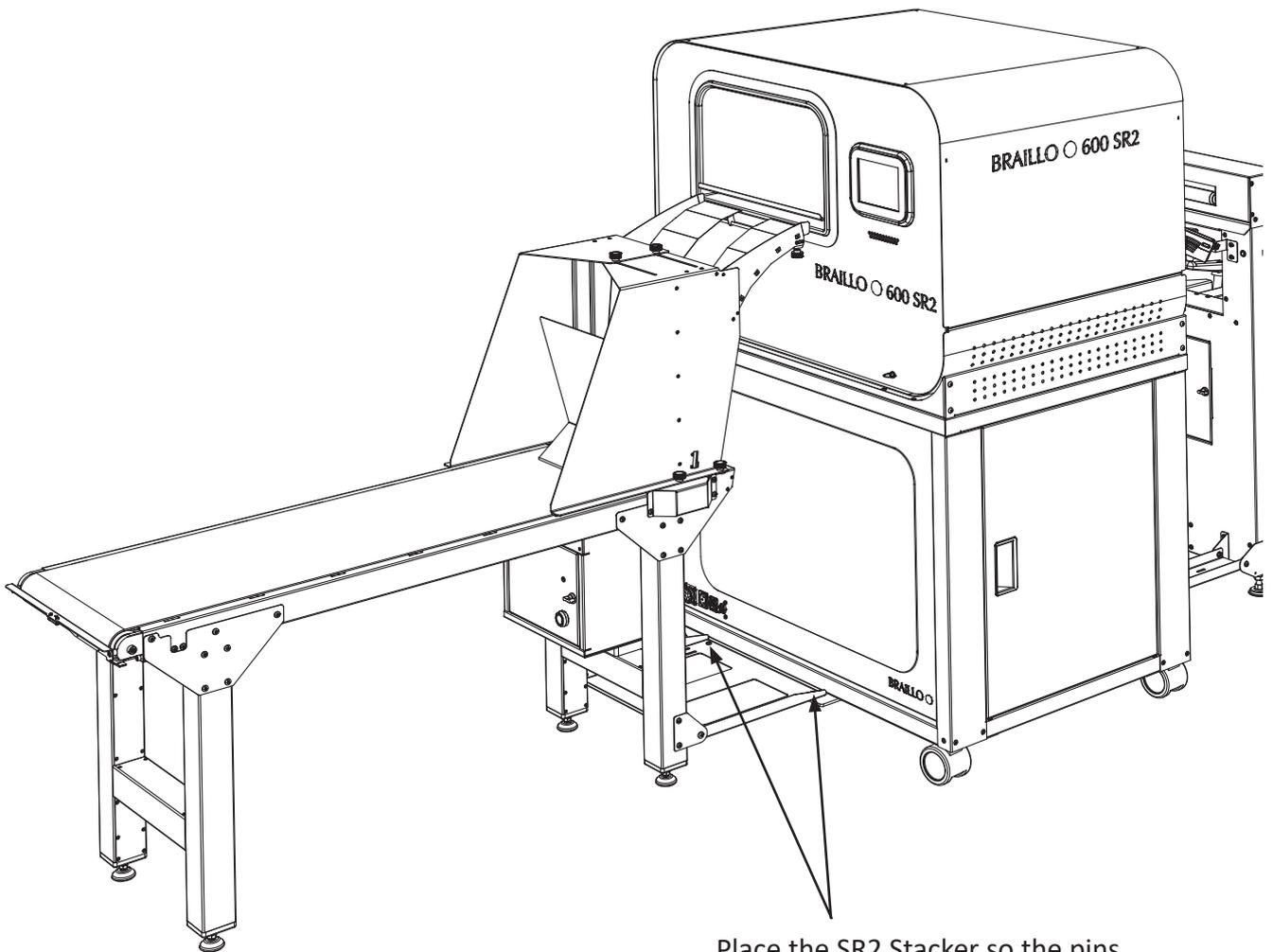
Place the SR2 Stacker so the pins will fit into the guide holes in the plate
