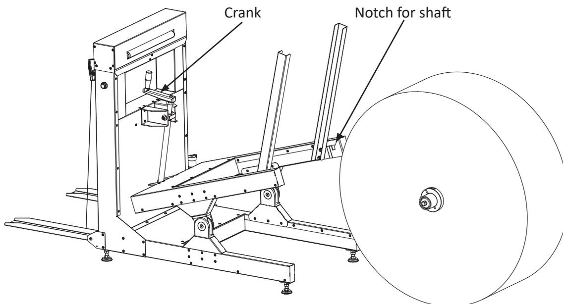
When the roll is lifted above the floor, place the friction bar between the guides, so it rests on top of the roll.
