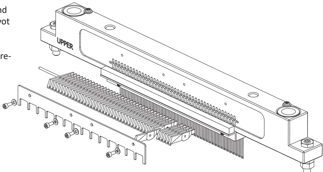
Note! When putting the short pivot arms back into the beam, be sure that the printing pins are hanging vertically like in the figure. This is to make room for the short pivot arm.
