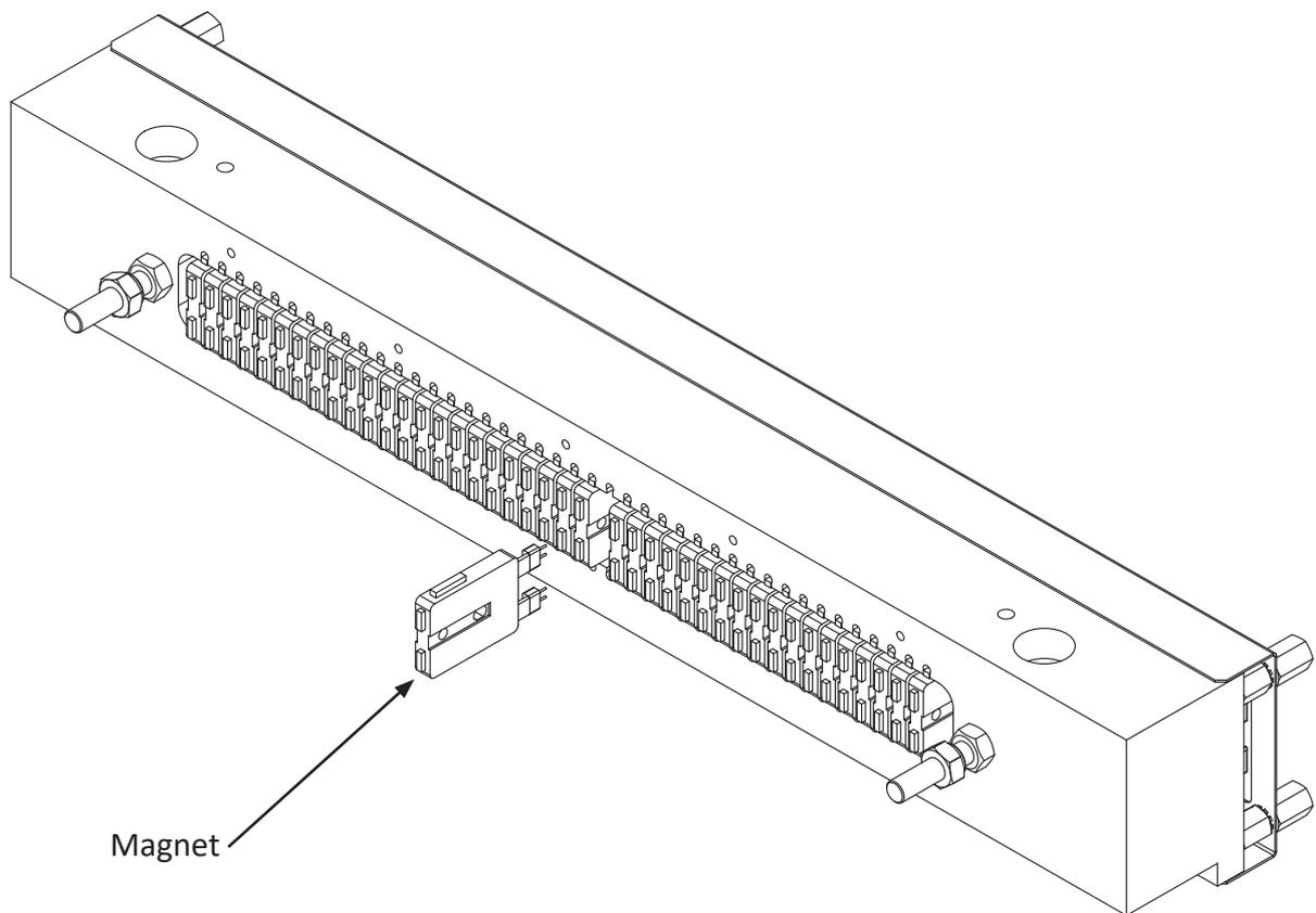
Step 3. Check the magnets internal resistance if you have an ohm-meter available. The resistance should be from 185 ohm to 240 ohm. Any value outside this range indicates a defect magnet.
