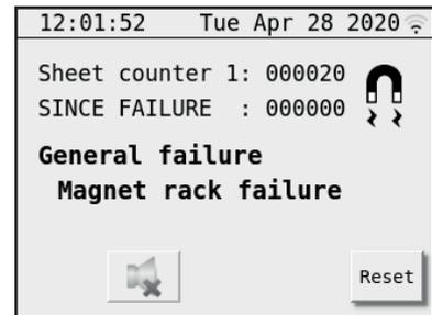
When trying to print after a defect magnet is found and replaced, the display will still show the magnet symbol in the top right hand corner. This is because you have to reset the magnet failure.
