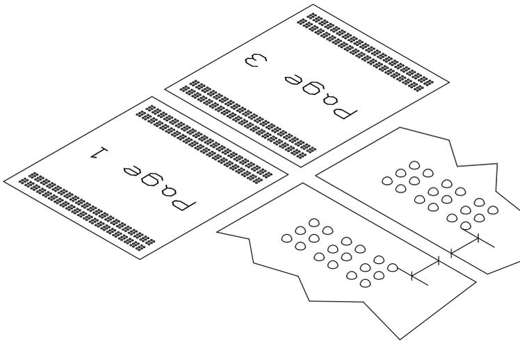
If the cutter calibration is correctly adjusted, the cut should be placed on the sheet like shown in the figure to the left. The distance from the cut to the braille text will be the same on both sides of the cut.
