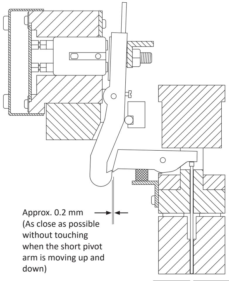
The gap between the long and the short pivot arm should be approximately 0.2 mm. When adjusting this, make sure that the gap is even for all the pivot arms and the same on both ends of the magnet rack.
