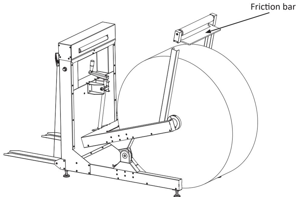
Thread the paper end in under the correction roll and then over it and towards the printer.
