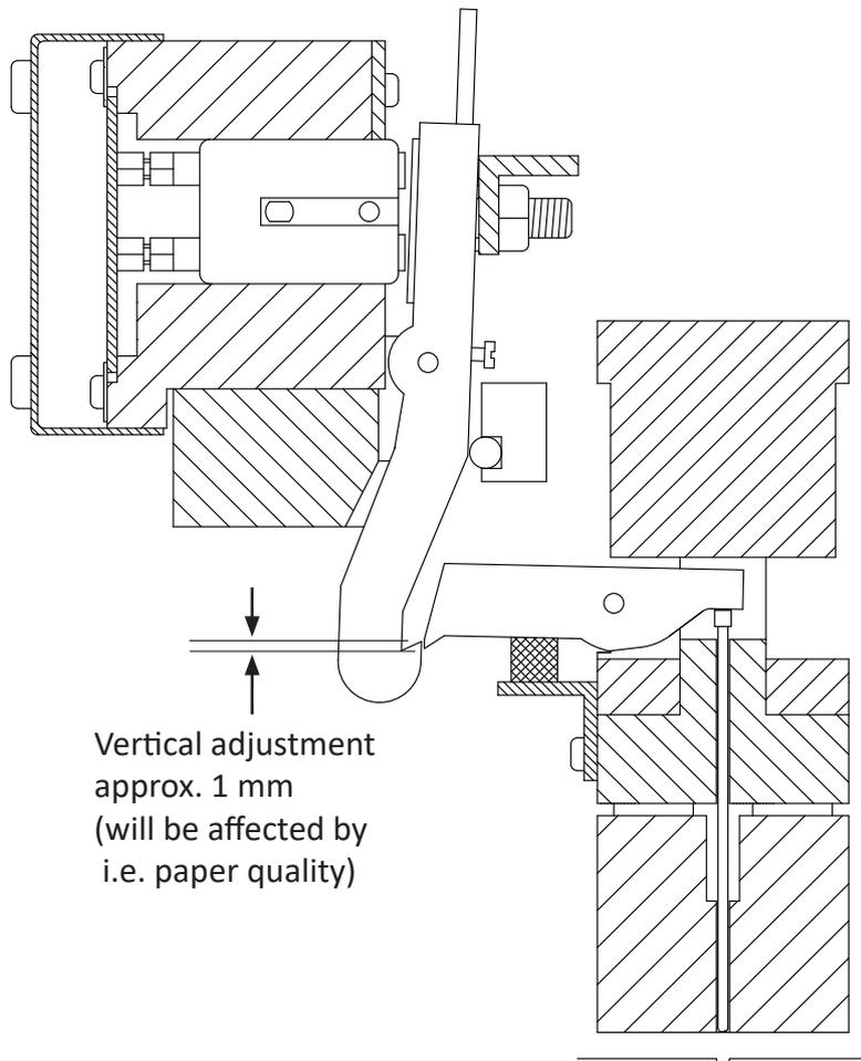
The vertical adjustment of the magnet rack sets the pressure of the printing pins when making dots.
