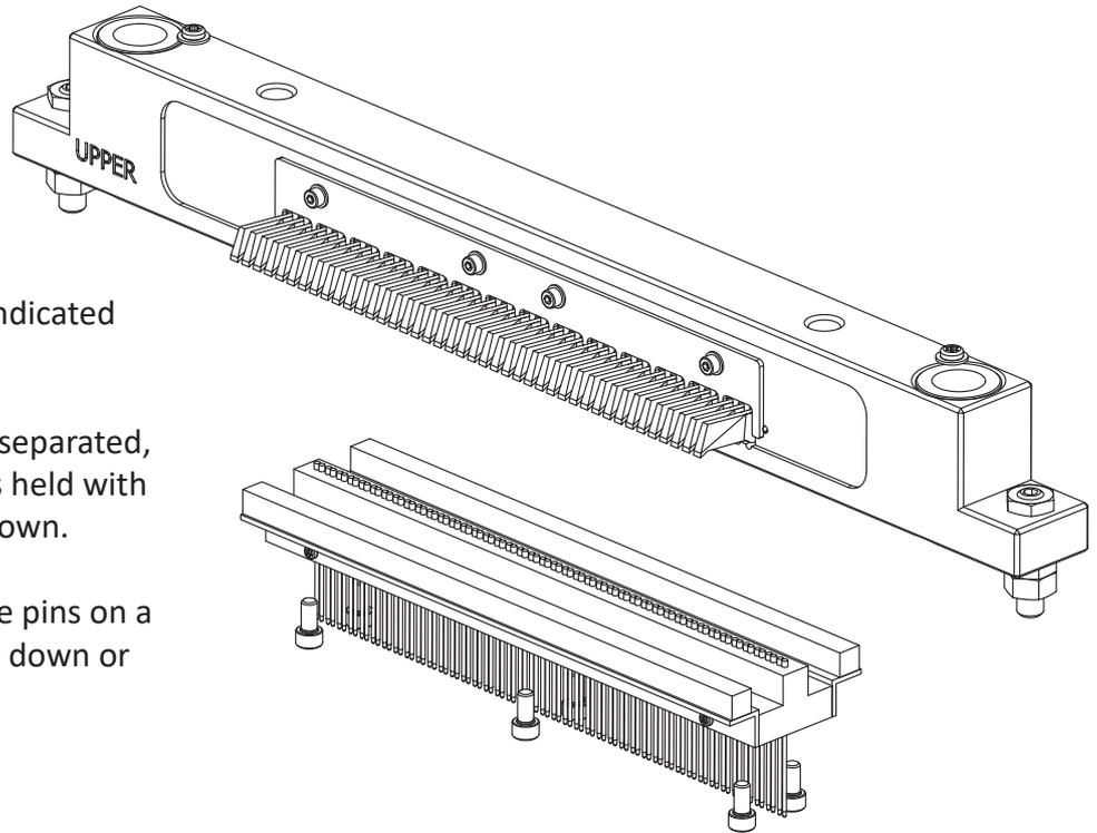
Now the defect printing pin can be replaced.
