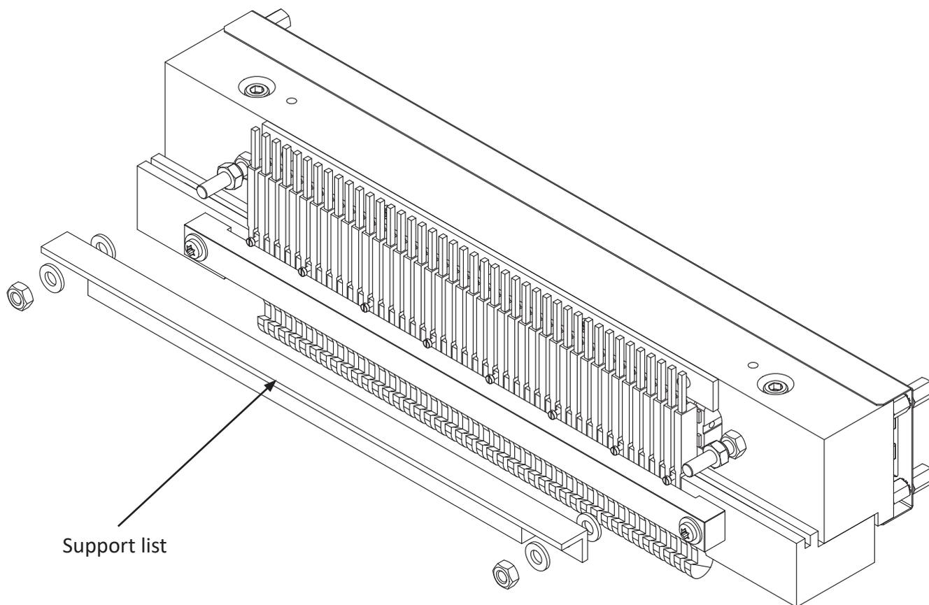
Step 2. Remove the two screws on the silicone string holder, and then remove the holder.
