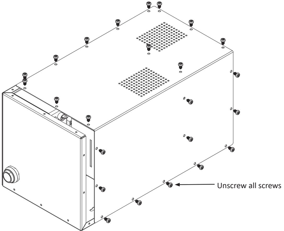
To get more room to inspect and replace the fuses, it is best to move the power supply a little out of the way. This can be done without disconnection the wires. See figure below:
