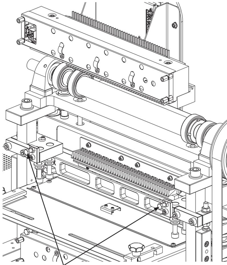
Pull back against these positioning screws on both ends
