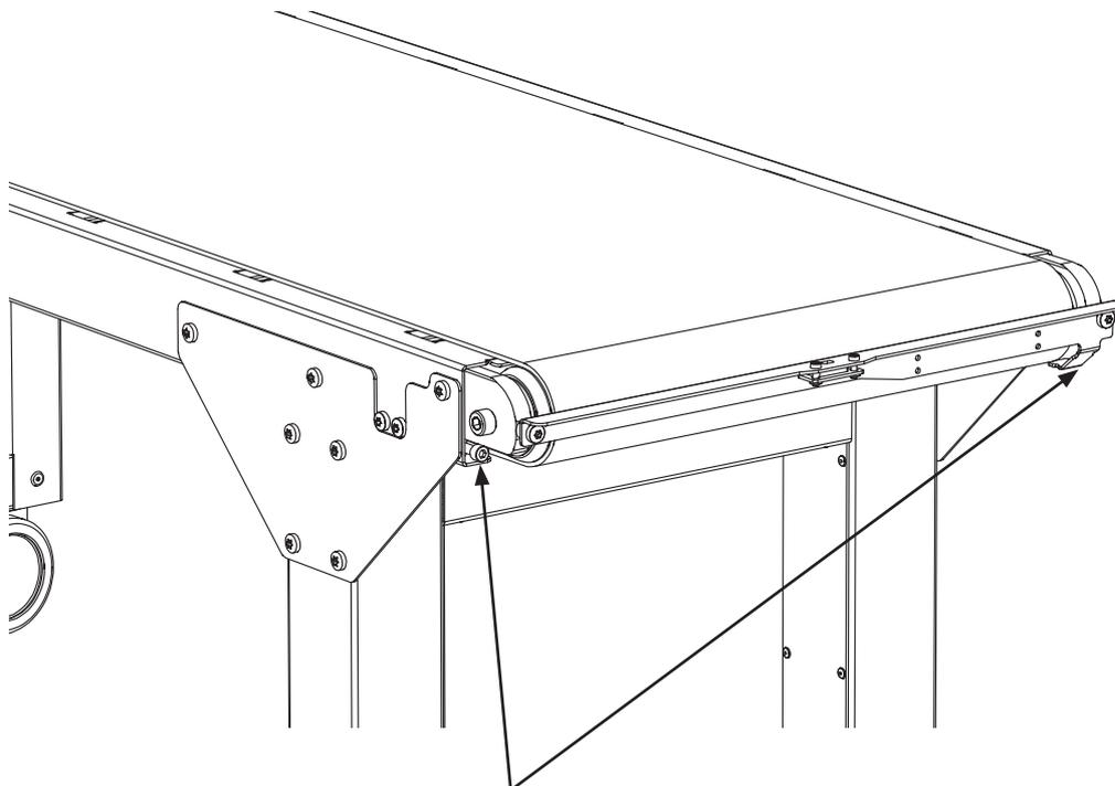
Conveyor belt tension adjustment screw
