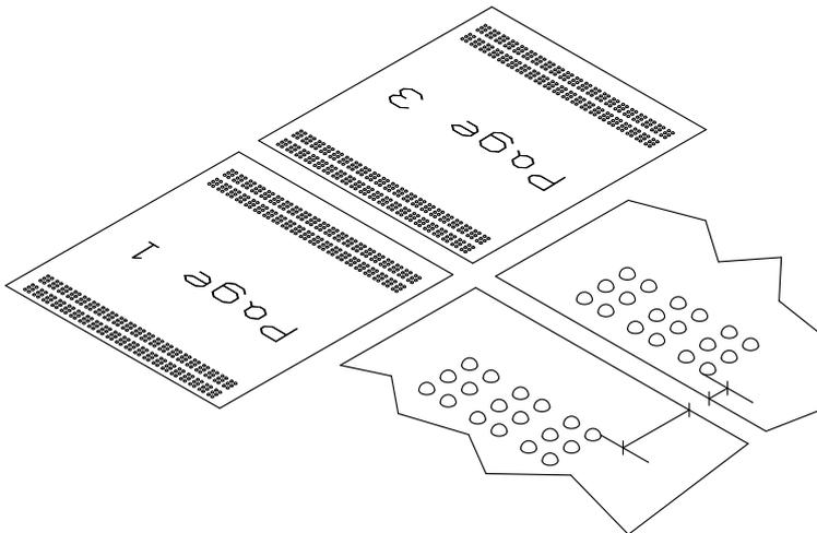
If the cutter calibration is adjusted too high, the cut will be placed nearer to the printed text on the starting edge of the paper.
