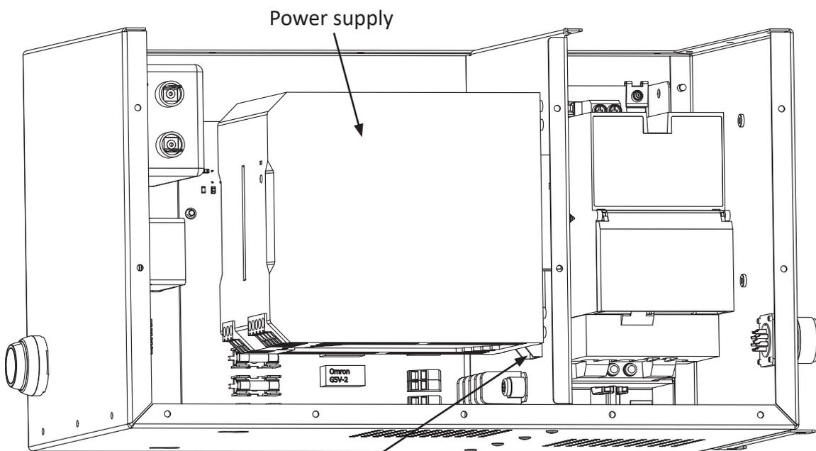
To release the power supply, place a screw driver here and pull the latch downwards
