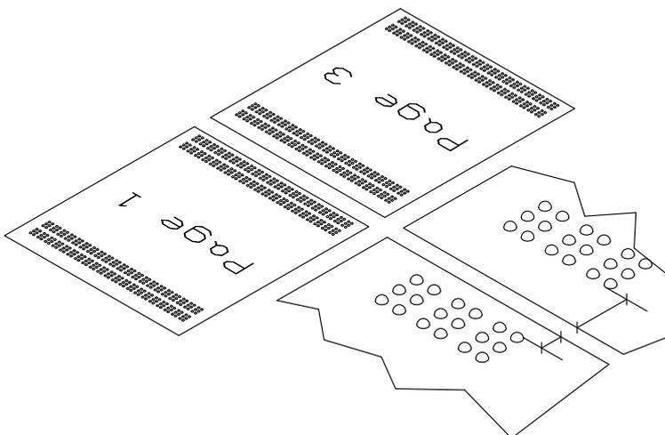
If the cutter calibration is adjusted too low, the cut will be placed further away from the printed text on the starting edge of the paper.
