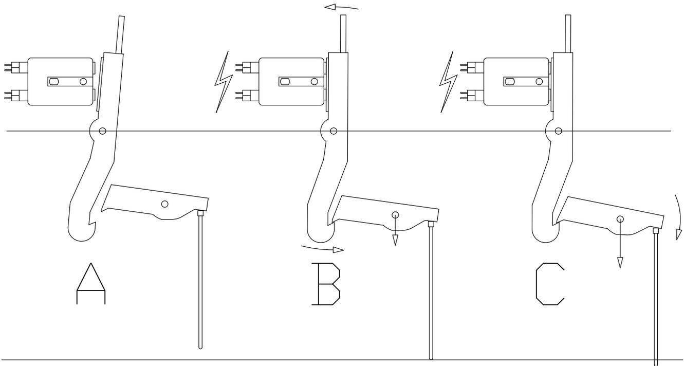
Figure A Shows the position on the pivot arm when the printer is not printing, and the magnet is not engaged.
