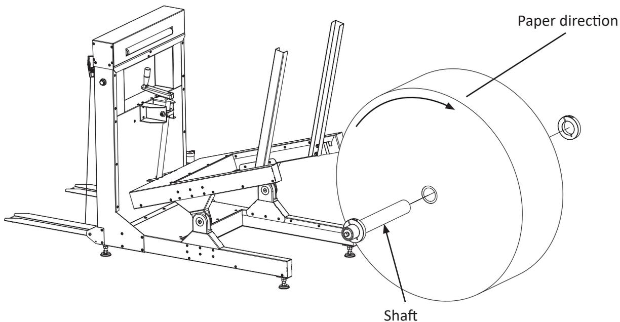
Use the crank to lower the two arms so it is lower than the shaft in the paper roll.
