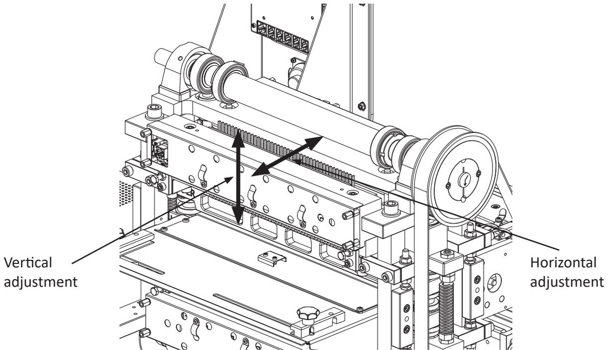
To be able to adjust the magnet rack correctly, it is necessary to put the printer in "printing position".
