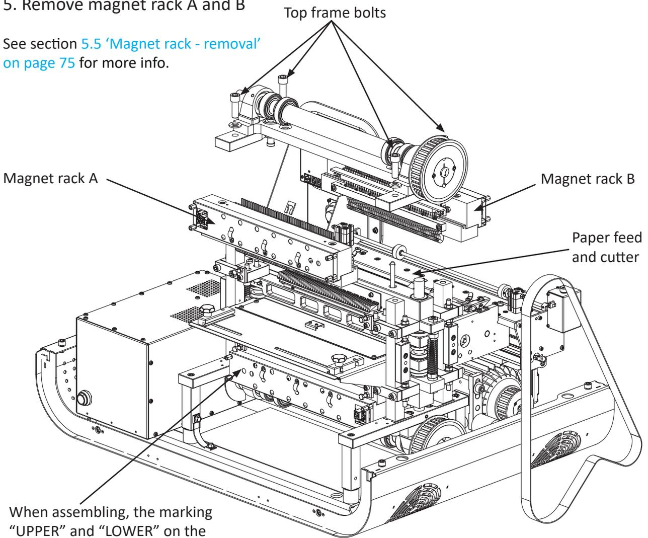
When assembling, the marking "UPPER" and "LOWER" on the paper shoes and beams, must be facing this side
