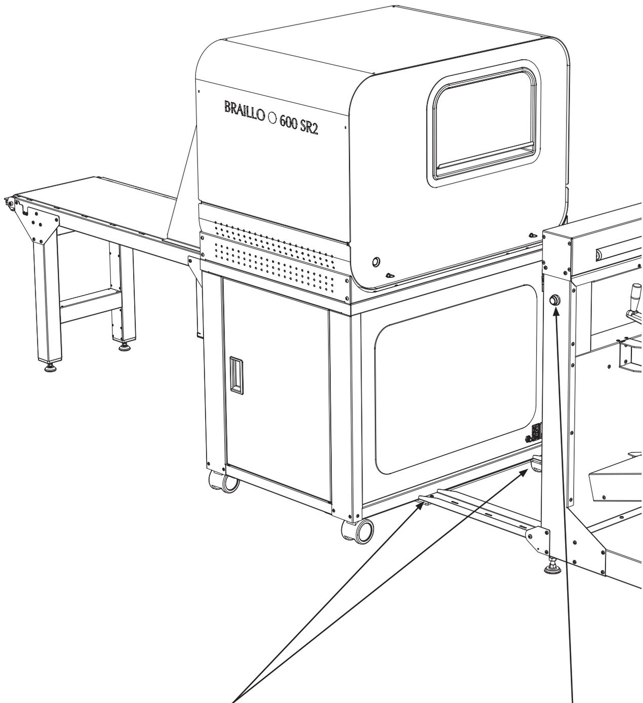
Place the Roll Unwinder so the pins will fit into the guide holes in the plate on the printer
