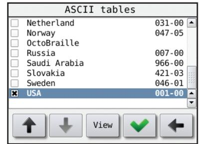
It is also possible to view the translation between characters and dots in the different ASCII tables by pressing the “View” button. Then a list like shown on the right will appear. Use the up and down arrows to scroll the list.
