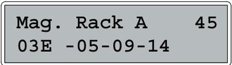
If there is detected one or more defect magnet(s) -when the printer is turned on, -when pressing reset, -or while the printer is running, this message will appear on the display. For more information - see chapter 3.5 "Selftest on magnets".
